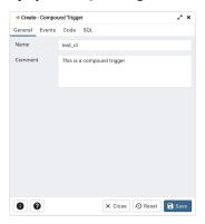
Use the fields in the *General* tab to identify the compound trigger:
