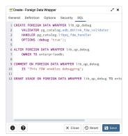
The example creates a foreign data wrapper named  $lib\_qp\_debug$  that uses pre-existing validator and handler functions,  $dblink\_fdw\_validator$  and  $libpg\_fdw\_handler$ . Selections on the Options tab set debug equal to true. The foreign data wrapper is owned by postgres.
