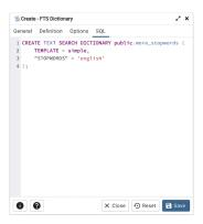
The example shown demonstrates creating a custom dictionary named *more\_stopwords* which is based on the simple template and is configured to use standard English.
