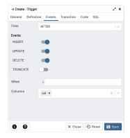
Use the fields in the *Events* tab to specify how and when the trigger fires:
