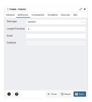
Use the fields in the *Definition* tab to add parameters for the column. (Fields are disabled if inapplicable.)
