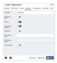
Use the fields in the *Options* tab to describe or modify the action of the trigger function:
