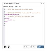
Use the *Code* field to specify the code for the five timing events *BEFORE STATEMENT*, *AFTER STATEMENT*, *BEFORE EACH ROW*, *AFTER EACH ROW*, *INSTEAD OF EACH ROW* that will be invoked when the compound trigger fires. Basic template is provided with place holders.
