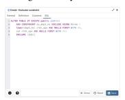
The example shown demonstrates creating an exclusion constraint named *ex\_dept\_no*. The constraint uses a btree index.
