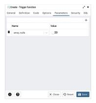
Use the fields in the *Parameters* tab to specify settings that will be applied when the trigger function is invoked. Click the *Add* icon (+) to add a *NamelValue* pair to the table below.
