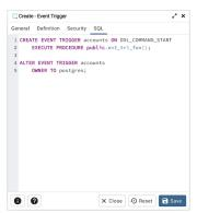
The command creates an event trigger named accounts that invokes the procedure named evt\_tri\_fun.
