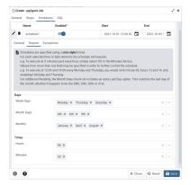
Use the fields on the *Repeat* tab to specify the details about the schedule in a cron-style format. The job will execute on each date or time element selected on the *Repeat* tab.
