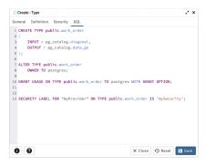
The example shown demonstrates creating a data type named *work\_order*. The data type is an enumerated type with three labels: new, open and closed.
