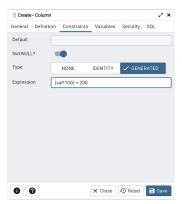
Use the following fields to create *GENERATED* column. Generated columns are applicable for PG/EPAS version 12 and above.
