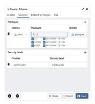
Use the Security tab to assign privileges and security labels for the schema.
